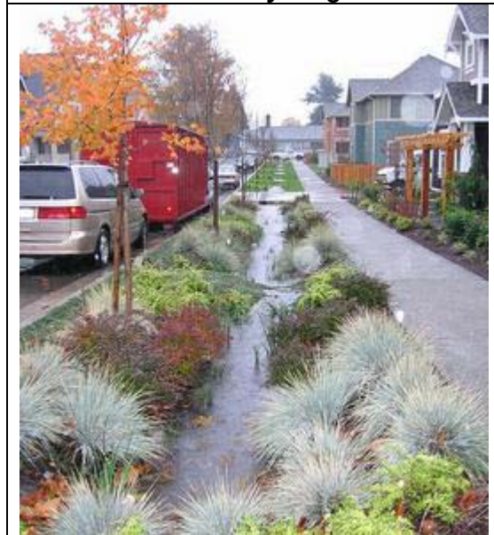
Figure 3.2.6. Open drainage applied in a medium density neighbourhood
