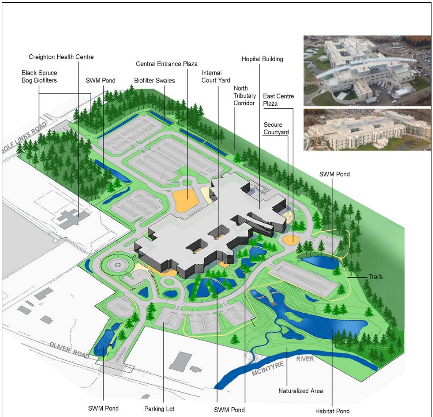
Figure 2.9.5 Institutional building – integrated stormwater management and landscaping plan
