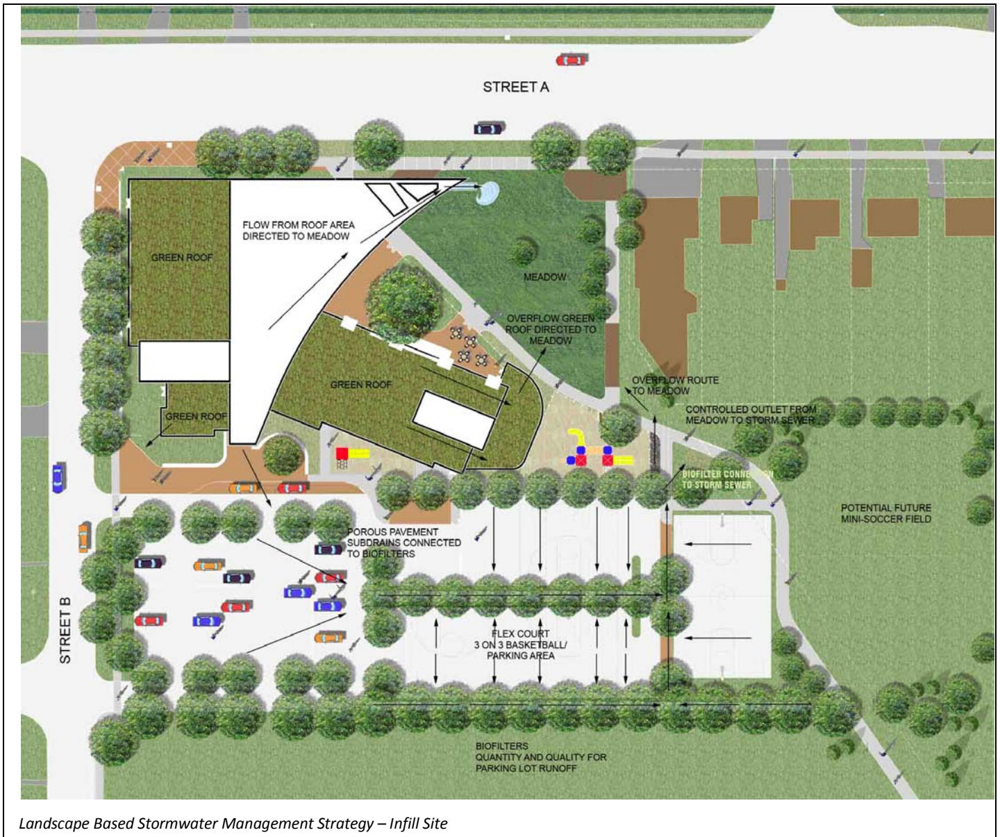
Figure 2.9.7 Landscape-based stormwater management strategy – infill site
