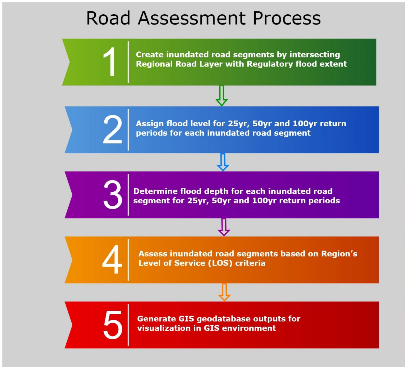
FIGURE 3.7 THE HIGH-LEVEL FLOWCHART OF OVERALL WORKFLOW FOR THE ROAD ASSESSMENT
