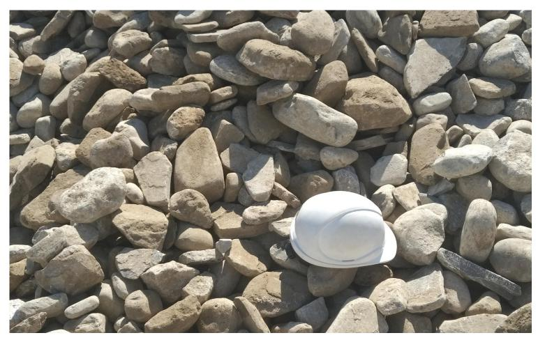
Example of a complete cobble revetment at Bluffer's Park (left), example of cobble material with a hard hat for scale (right).
