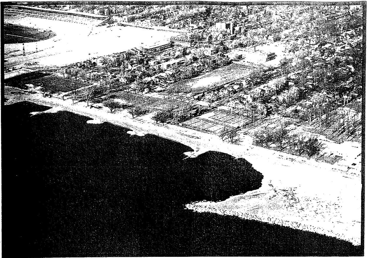
EASTERN BEACHES: THE POPULAR BOARDWALK WAS DESTROYED IN THIS AREA IN 1973. SHORELINE PROTECTION CONSTRUCTED BY THE AUTHORITY IN 1979 INCLUDED A WIDE PROTECTIVE BEACH. (PHOTO 3)
