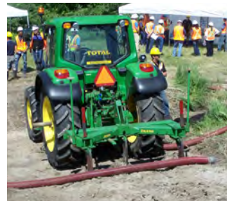
From left to right: Chisel plow (Source: J. Balousek); Subsoiler with roller (Source: Agrional); LGP rated tractor with subsoiler (Source: TRCA).
