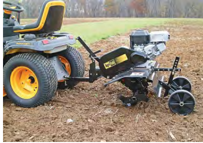
Figure 5.1 Examples of rototilling equipment appropriate for decompacting subsoil.
