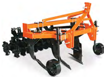
Figure 5.2 Examples of subsoiling equipment appropriate for decompacting subsoil
