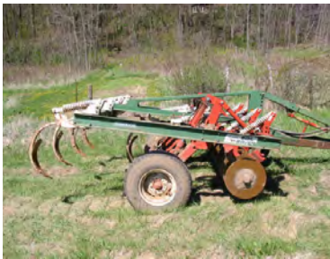
Figure 5.2 Examples of subsoiling equipment appropriate for decompacting subsoil
