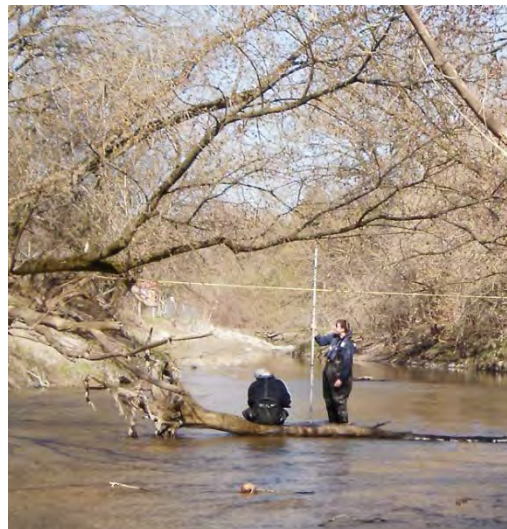
Figure 9: TRCA staff measuring the “control” cross-section of a stream at a RWMP site.
