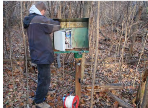
Figure 11: TRCA staff checking equipment at a groundwater well monitoring site.
