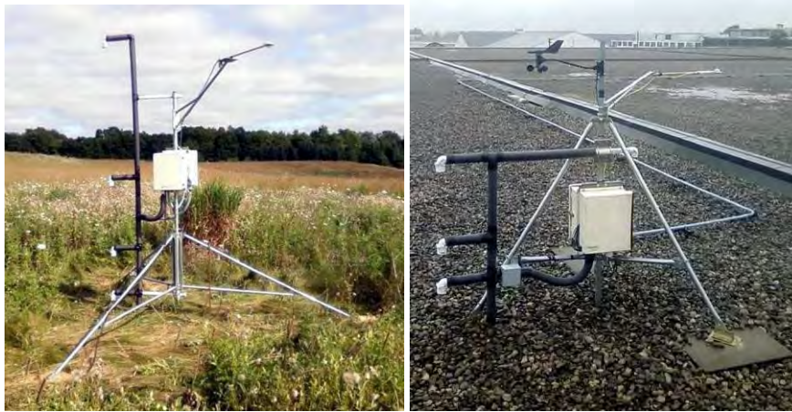
Figure 20: Automated Bowen Ratio Energy Balance system used to determine “actual” evapotranspiration values, located at Kortright Conservation Area (left) and Downsview Park (right).
