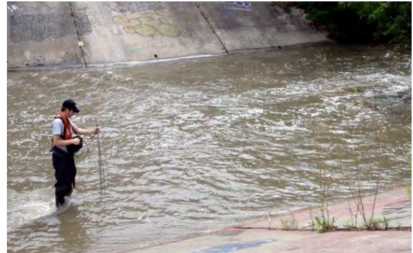
Figure 12: TRCA technician conducting flow metering using Area-Velocity Method
