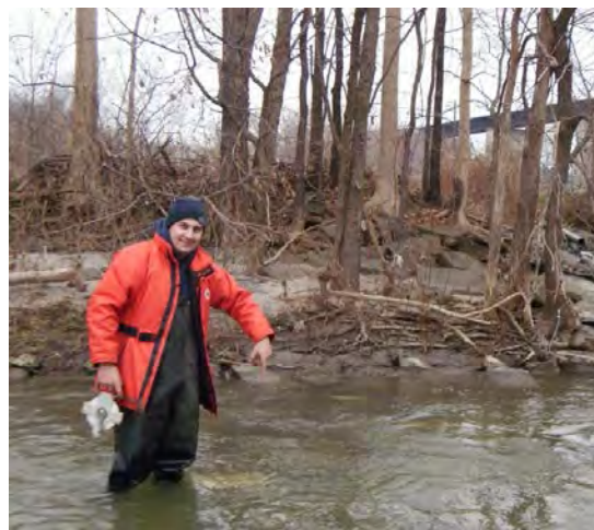
Figure 7: TRCA staff installing a year round water temperature logger attached to a cement block.
