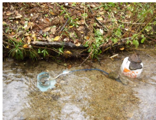
Figure 33: Seepage meter with tubing attached.
