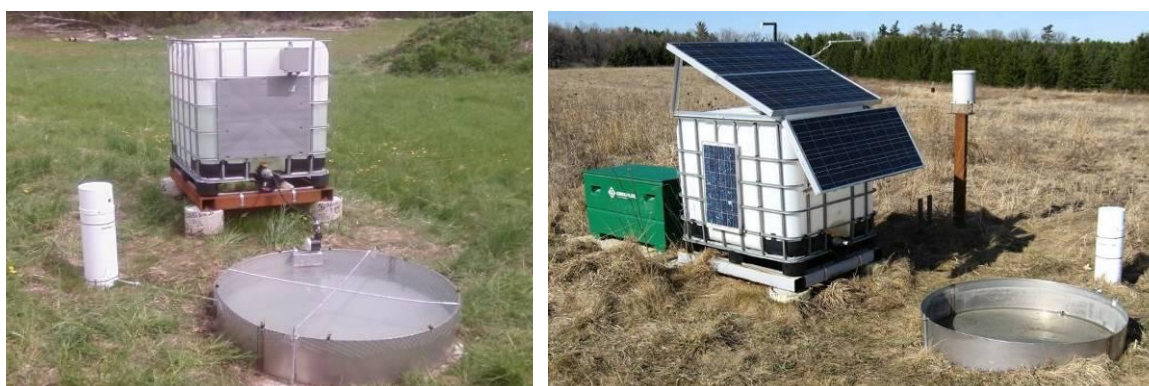
Figure 45: Automated evaporation pans located at Glenn Haffey Conservation Area (left) and Kortright Conservation Area (right). Glenn Haffey station depicting operational setup and Kortright station prior to spring deployment.
