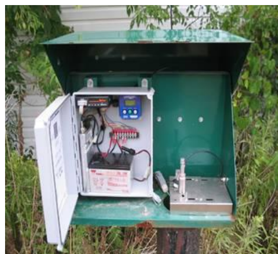
Figure 32: PGMN well with telemetry equipment and dedicated pump installed.
