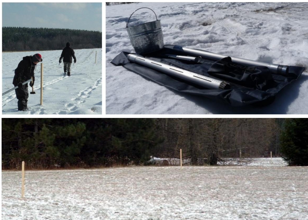
Figure 37. Snow course sampling: Albion Hills CA (upper left), Mount Rose sampling kit (upper right), and Greenwood CA 3 of 10 sample points (above).
