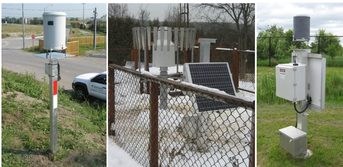
Figure 36. Various precipitation gauges. From left to right: 3-season “stand-alone” rain gauge, a 4-season RT weight gauge with windscreen, and a 4-season heated rain gauge.
