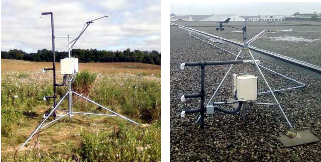
Figure 48. Automated Bowen Ratio Energy Balance system used to determine “actual” evapotranspiration values, located at Kortright Conservation Area (left) and Downsview Park (right).
