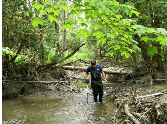
Figure 28. Conducting a cross-sectional profile survey
